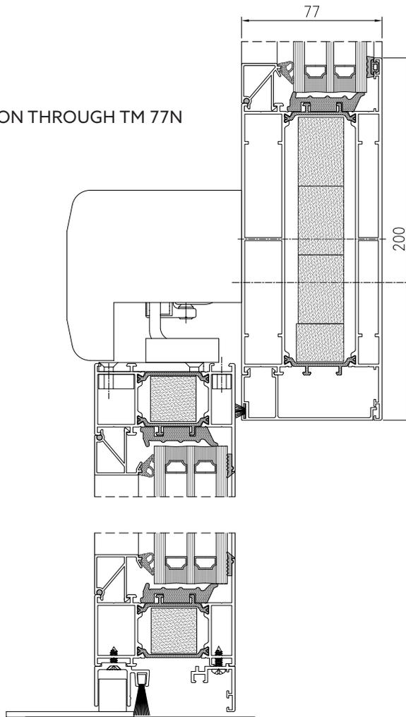
CROSS SECTION THROUGH DOOR LIMITER AT THE JOINT WITH THE WALL OF TM 77N PROFILE
